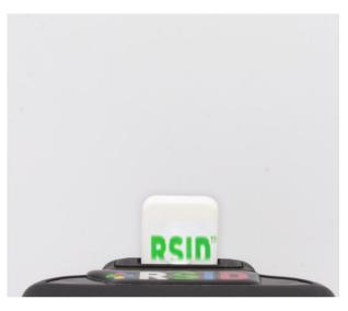
**Caution:** The cassette must be inserted as shown, right side up and facing you or test will read INVALID or give an inaccurate result.
